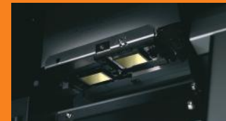
Dual print heads in staggered formation.
