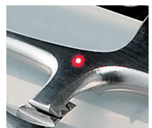
Accurately set the correct marking location with the built-in laser pointer
